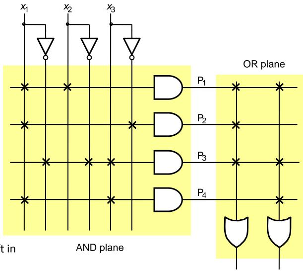
x marks the connections left in place after programming
