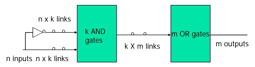
Programmable AND array + programmable OR array
