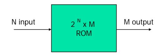
Address: N bits; Output word: M bits
