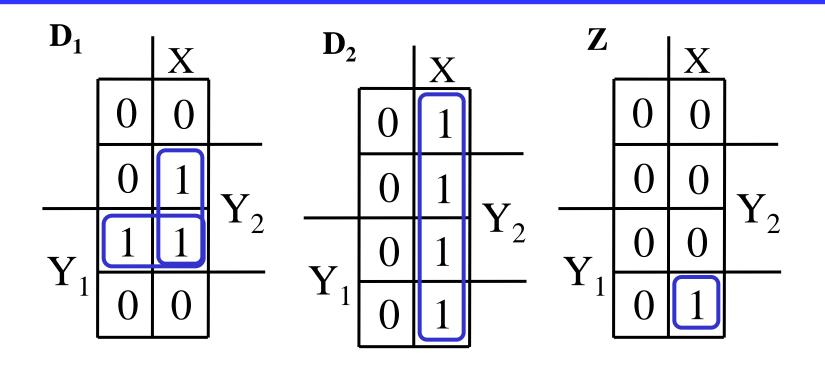
$$\begin{aligned} D_1 &= Y_1 Y_2 + X Y_2 & \text{Gate Input Cost} &= 9 \\ D_2 &= X & \text{Select this state assignment to} \\ Z &= X Y_1 \overline{Y}_2 & \text{complete the design} \end{aligned}$$
