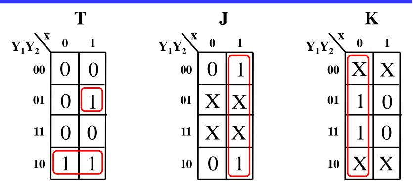
$$T = Y_1 \overline{Y}_2 + X \overline{Y}_1 Y_2, \quad J = X, \quad K = \overline{X}$$
