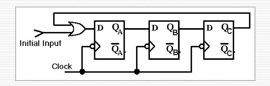
In Class: Build a ring counter using electronics simulation tools
