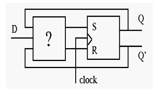
We need to design the circuit to generate the triggering signals S and R as functions of D and Q.
