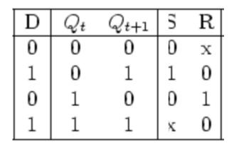
The desired signal S and R can be obtained as functions of D and Q current FF state from the Karnaugh maps:
