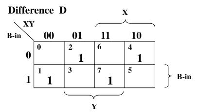
S = X'Y'(B-in) + XY'(B-in)' + XY'(B-in)' + XY(B-in) $S = X \oplus Y \oplus (C-in)$
