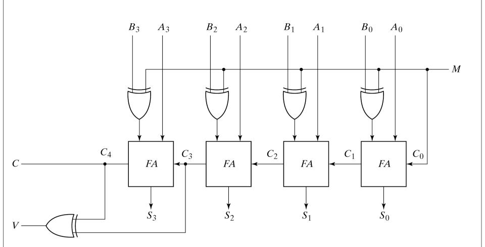
Fig. 4-13 4-Bit Adder Subtractor
