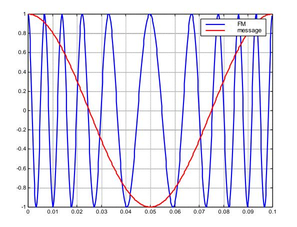
Inst.frequency Moves with the Message amplitude
