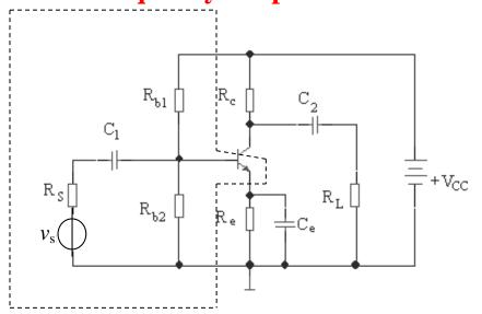
At low frequencies,  $C_1$ ,  $C_2$  are an open circuit and the gain is zero. Thus  $C_1$  has a high pass effect on the gain, i.e. it affects the lower cutoff frequency of the amplifier.
