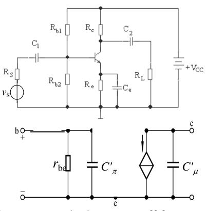
At high frequencies,  $C_1$ ,  $C_2$   $C_e$  are all short circuit.
