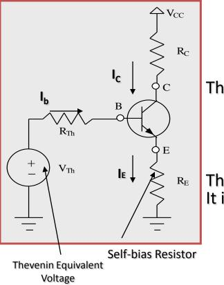
Applying KVL through input base circuit
