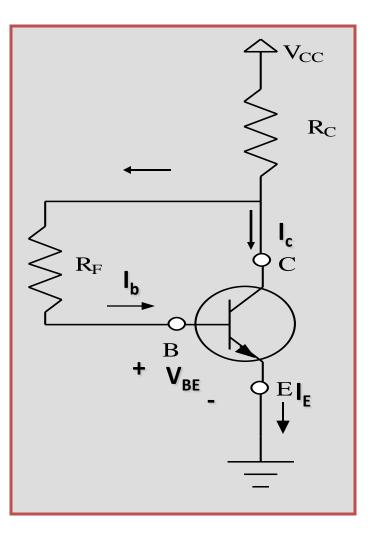
This configuration employs negative feedback to prevent thermal runaway and stabilize the operating point. In this form of biasing, the base resistor  $R_F$  is connected to the collector instead of connecting it to the DC source V<sub>cc</sub>. So any thermal runaway will induce a voltage drop across the Rc resistor that will throttle the transistor's base current.
