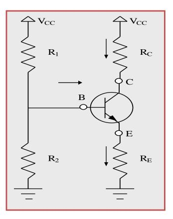
To find the stability of this circuit we have to convert this circuit into its Thevenin's Equivalent circuit
