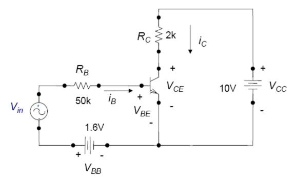
Likewise, we can write KVL around the collector circuit.
