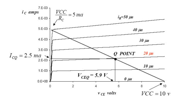
Now that we have the Q-point for the base circuit, let's proceed to the collector circuit.
