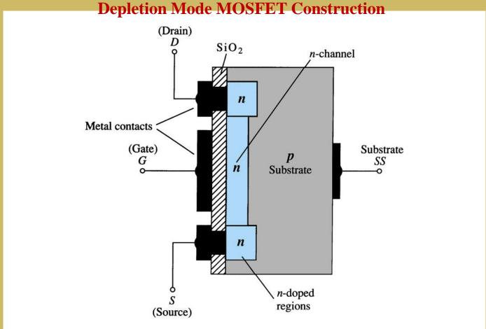
The Drain (D) and Source (S) leads connect to the to n-doped regions
