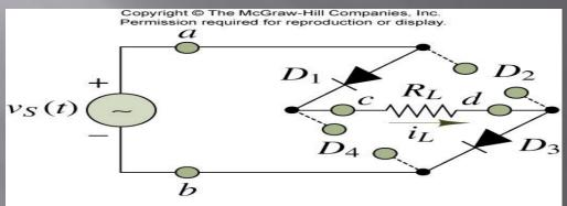
During the positive half-cycle of  $v_S(t)$ ,  $D_1$  and  $D_3$  are forward-biased and  $i_L = v_S(t)/R_L$  (ideal diodes).
