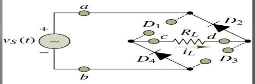
During the negative half-cycle of  $v_S(t)$ ,  $D_2$  and  $D_4$  are forward-biased and  $i_L = -v_S(t)/R_L$  (ideal diodes).
