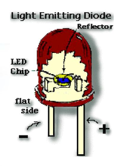
When sufficient voltage is applied to the chip across the leads of the LED, electrons can move easily in only one direction across the junction between the p and n regions.
