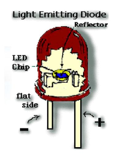
Each time an electron recombines with a positive charge, electric potential energy is converted into electromagnetic energy.
