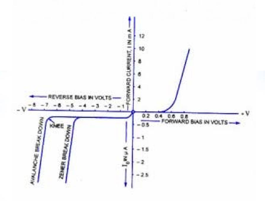
The critical value of the voltage, at which the breakdown of a P-N junction diode occurs is called the *breakdown voltage*.
