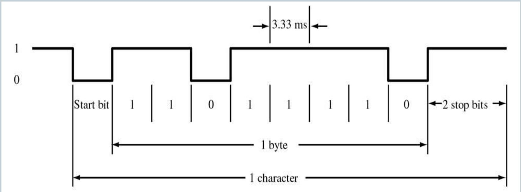
a) Serial Data transmitted at proper rate
