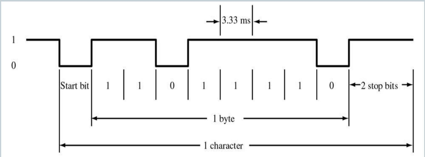
a) Serial Data transmitted at proper rate
