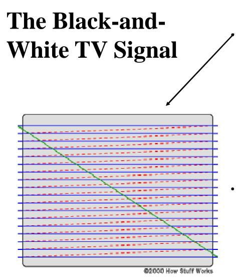
The blue lines represent lines that the electron beam is "painting" on the screen from left to right, while the red dashed lines represent the beam flying back to the left. When the beam reaches the right side of the bottom line, it has to move back to the upper left corner of the screen, as represented by the green line in the figure. When the beam is "painting," it is on, and when it is flying back, it is off so that it does not leave a trail on the screen.
