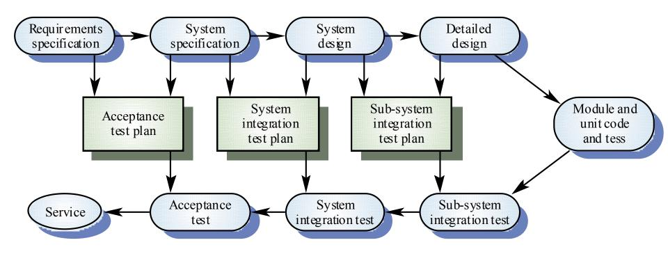
This diagram shows how test plans should be derived from the system specification and design.
