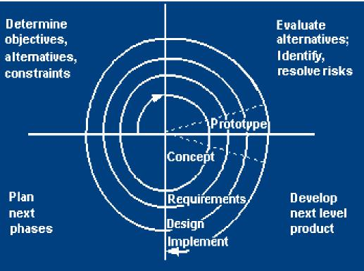
Adds risk analysis, and 4gl RAD prototyping to the waterfall model
