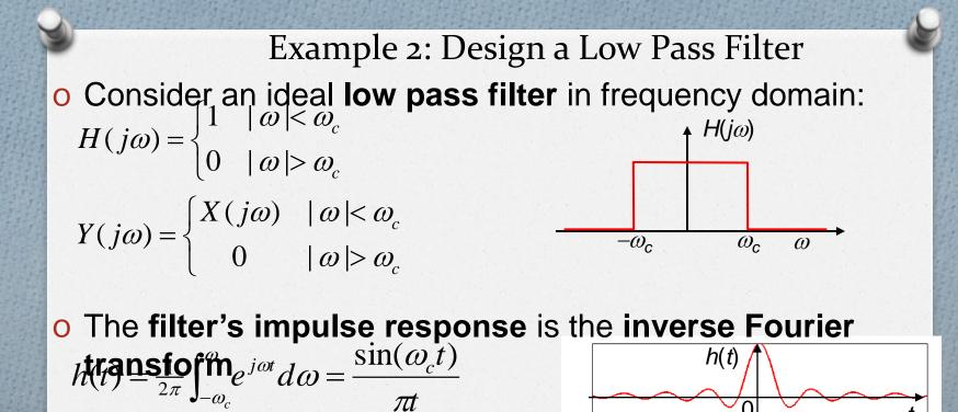
o which is an ideal low pass CT filter. However it is noncausal, so this cannot be manufactured exactly & the time-domain oscillations may be undesirable • We need to approximate this filter with a causal system such as  $1^{OV(t)}$  order (LTL system impulse response { h(t),
