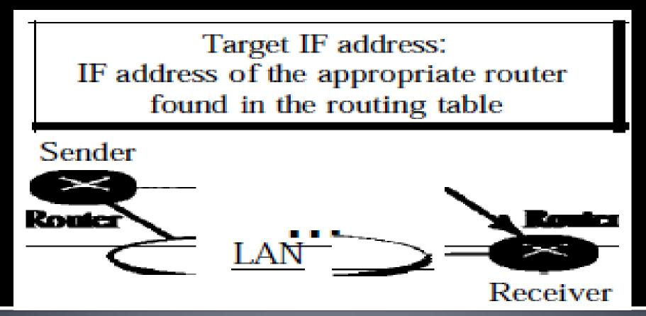
The sender is a router that has received a datagram destined for a host on another network. It checks its routing table and finds the IP address of the next router. The IP address of the next router becomes the logical address that must be mapped to a physical address
