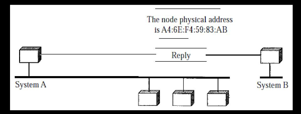
Every host and router on the n/w receives and process the ARP request packet. But only B recognizes its IP address and send back ARP response packet. Which contains the IP and physical address of receiver(B) .this packet delivered only to A using A's physical address in ARP request packet.
