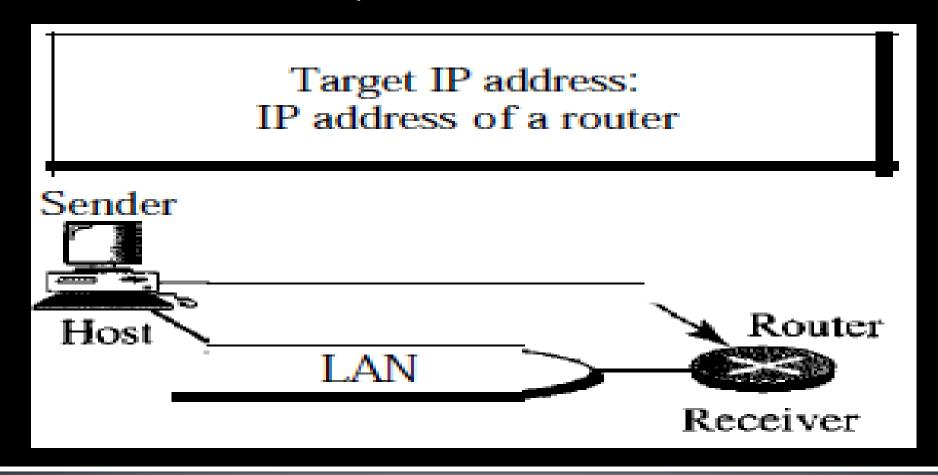
In this case, the host looks at its routing table and finds the IP address of the next hop (router) for this destination. If it does not have a routing table, it looks for the IP address of the default router. The IP address of the router becomes the logical address that must be mapped to a physical address
