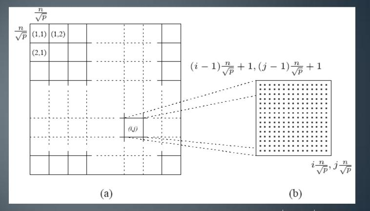
(a) Matrix  $D^{(k)}$  distributed by 2-D block mapping into  $\sqrt{p} \times \sqrt{p}$  subblocks, and (b) the subblock of  $D^{(k)}$  assigned to process  $P_{i,i}$ .
