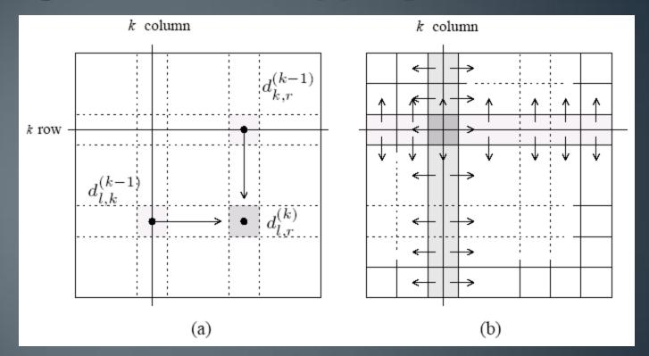
(a) Communication patterns used in the 2-D block mapping. When computing  $d_{i,j}^{(k)}$ , information must be sent to the highlighted process from two other processes along the same row and column. (b) The row and column of  $\sqrt{p}$  processes that contain the  $k^{th}$  row and column send them along process columns and rows.
