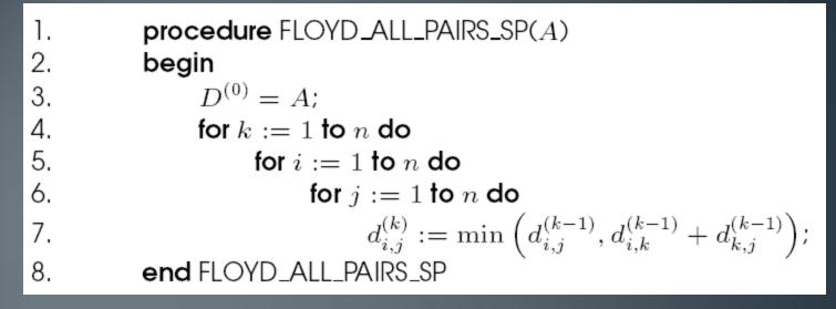
Floyd's all-pairs shortest paths algorithm. This program computes the all-pairs shortest paths of the graph G = (V,E) with adjacency matrix A.
