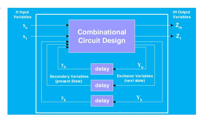
The <u>delay</u> elements can be viewed as providing short term memory for the sequential circuit.
