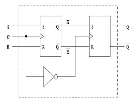
The left hand latch is called the master and the right hand latch the slave.
