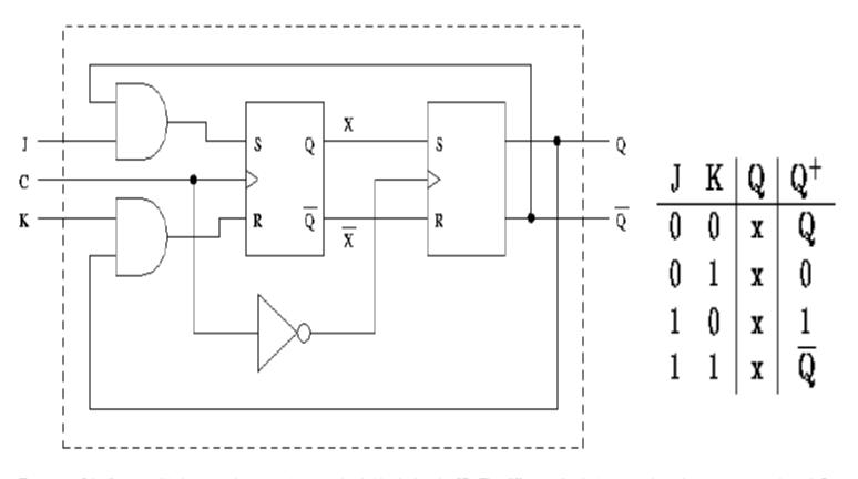
For three of the four possible input combinations the operation is identical to the SR. The difference lies in the case where the two inputs are both 1. In
