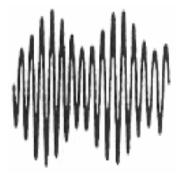
The input to the diode detector from the last IF amplifier
