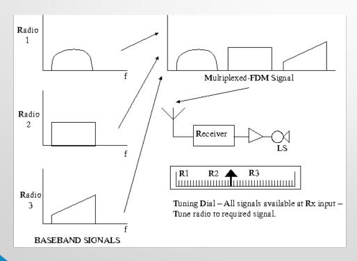
Frequency Divison Multiplexing composite signal spectrum **ISCN** Sec.2 0 J<sub>SC1</sub> Message  $B_{SCN}$  $B_{SC1}$  $B_{SC2}$ signals  $\rightarrow m_1(t)$ Demodulator > LPF BPF Modulator LPF LPF BPF Demodulator Modulator LPF Channel | Demodulator - LPF  $m_{\rm K}(t) \longrightarrow$ BPF LPF Modulator ... ... FDM system Frequency Frequency block diagram synthesizer synthesizer Receiver Transmitter
