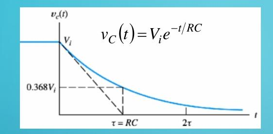
Exponential decay waveform RC is called the time constant. At time constant, the voltage is 36.89 of the initial voltage.
