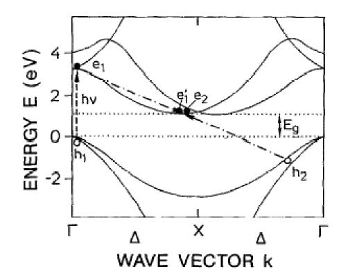
Many E-H pairs created by incident photon through impact ionization of hot carriers
