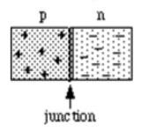
When sufficient voltage is applied to the <a href="https://doi.org/10.15">chip across the leads</a> of the LED, electrons can move easily in only one direction across the *junction* between the p and n regions.
