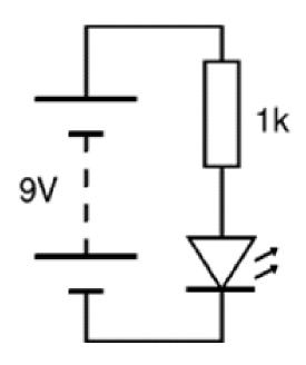
The energy (E) of the light emitted by an LED is related to the electric charge (q) of an electron and the voltage (V) required to light the LED by the expression: E = qV Joules.
