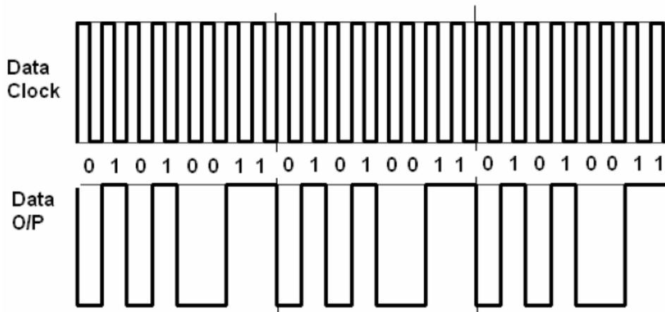
**Verify data O/P waveforms for other BCD inputs.**
