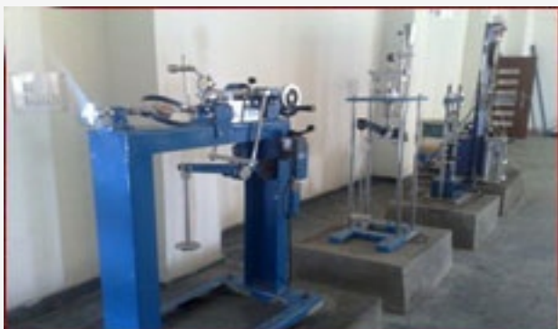
Soil Mechanics Lab showing apparatus for example: Direct Shear, Consolidation, Unconfined compression and Triaxial Tests
