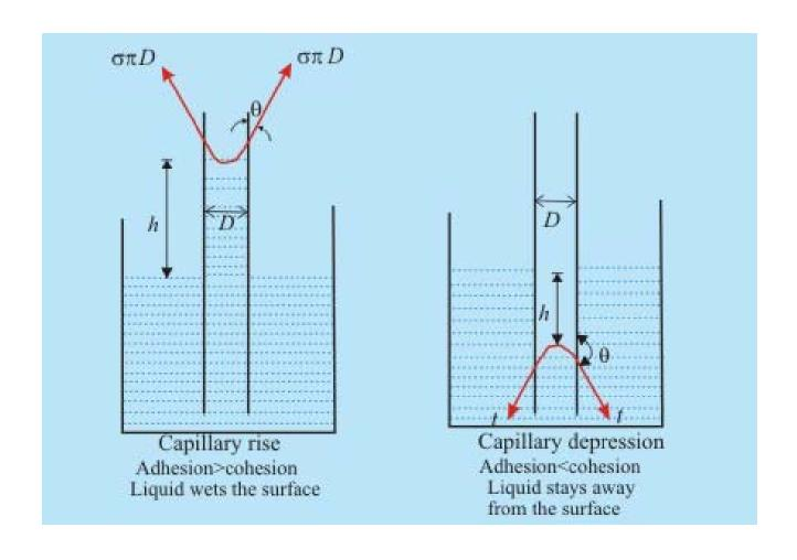
For pure water in contact with air in a clean glass tube, the capillary rise takes place with  $\theta = 0$ . Mercury causes capillary depression with an angle of contact of about  $130^{\circ}$  in a clean glass in contact with air. Since h varies inversely with D as found from Eq., an appreciable capillary rise or depression is observed in tubes of small diameter only.
