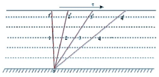
If a shear stress  $\tau$  is applied at any location in a fluid, the element 011' which is initially at rest, will move to 022', then to 033'. Further, it moves to 044' and continues to move in a similar fashion.
