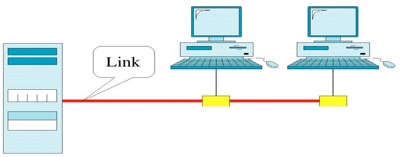
A **multipoint** (also called **Multidrop**) connection is one in which more than two specific devices share a single link.
