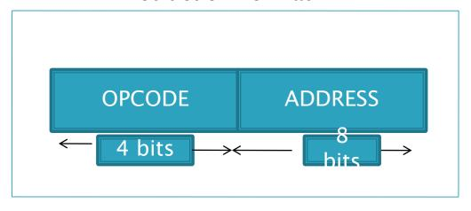
Opcode— (it stands for operation code). It indicates what operation is to be done .such as addition, subtraction, multiplication etc.
