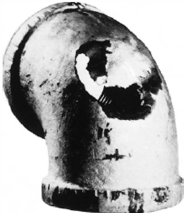
Figure 17.20 Impingement failure of an elbow that was part of a steam condensate line. (Photograph courtesy of Mars G. Fontana. From M. G. Fontana, Corrosion Engineering , 3rd edition. Copyright © 1986 by McGraw-Hill Book Company. Reproduced with permission.)
