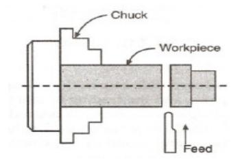
**Parting**: The parting or cutting off is the operation of cutting away a desired length of the workpiece, *i.e.*, dividing the workpiece in two or more parts.
