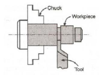
**Threading**: Threading is the act of cutting of the required form of threads on the internal or external cylindrical surfaces.
