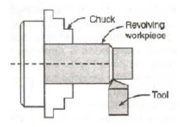
**Step Turning**: Step turning produces various steps of different diameters.
