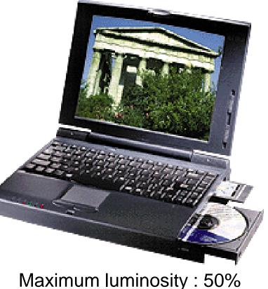
Maximum luminosity : 50% of CRT as 50% of light is blocked by the upper polarizer.
